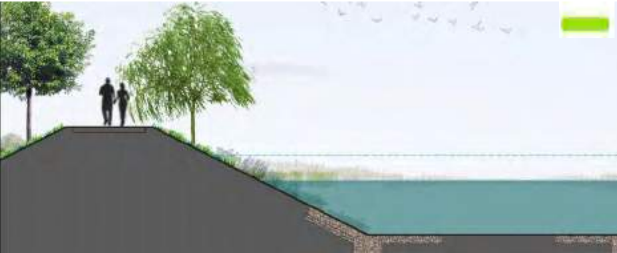
Bio-Engineered Erosion Control Embankment
