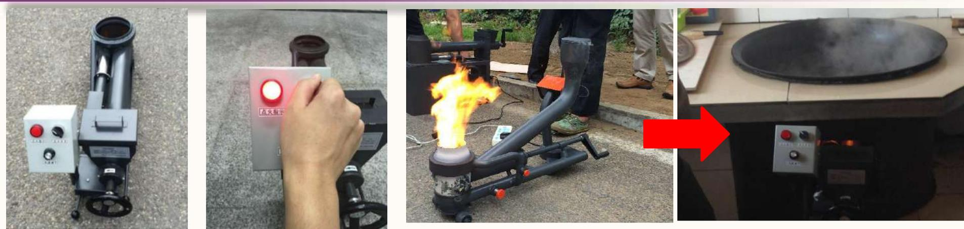
This burner can be integrated with existing facilities without changing the original operating mode and cooking habits, by manual feeding and reasonable semi-gasification combustion to achieve high performance of efficiency and emission.
