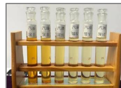
汽油国I至国VI油样 Gasoline sample from China I to VI
